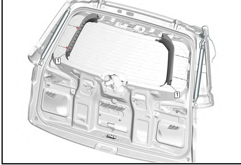
Liftgate Upper Side Trim Finish Panel (1) - Install - Liftgate Upper Side Trim Finish Panel Replacement
